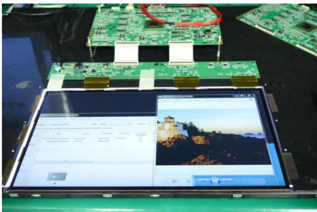
FIGURE 11 — 15.6" TFT-LCD prototype panel for 55" green UHD(4k) with Universal Column Driver ICs.
